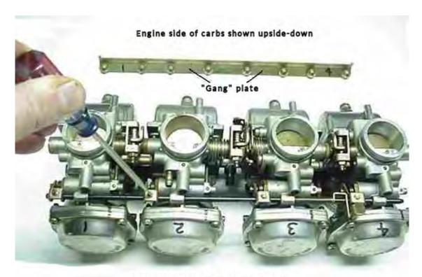
Loosening screws in preparation of removing Choke Actuation Rail.
