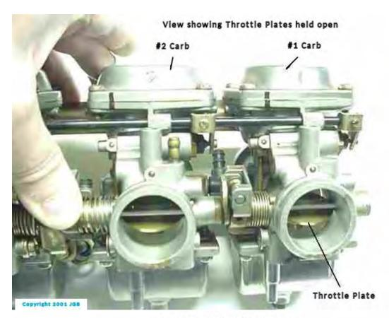
Throttle Valve (Slides) shown #1 down, #2 part way up.
