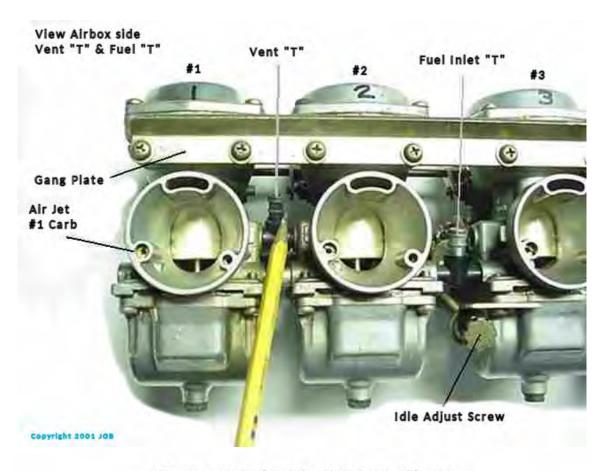
Vacuum port on #2 carb pointed out. This port goes to the fuel petcock small tube fitting.
