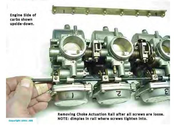
Engine side of carbs shown ready to separate, with choke rail (foreground) and "gang" plate removed (background)
