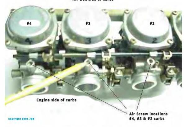
Engine side of carbs shown with Choke Rail pointed out.
