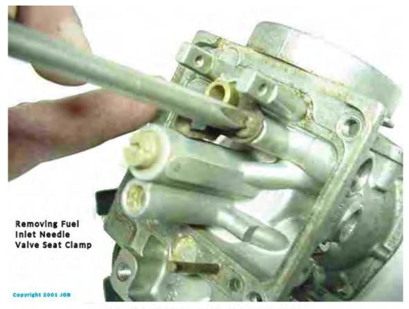
Removing Fuel Inlet Needle Valve Seat Clamp
